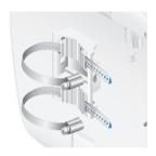
Wrap the Metal Straps around the pole. Use a 7 mm socket wrench to turn the screws clockwise and securely fasten the straps to the pole.
