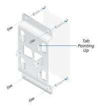
2. Insert the tabs of the *Wall-Mount Bracket* into the slots of the EdgePoint. Slide the EdgePoint down.
