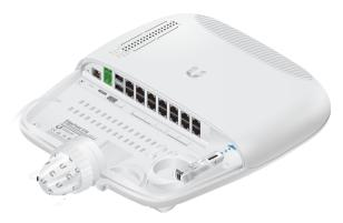
2. Feed the fiber optic cable through the *Cable Sleeve*, and remove the cable jacket from the fiber optic cable.
