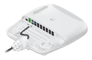
3. You can create a strain relief for any Ethernet cable by feeding a cable tie (not included) through the tie slot under the cable. Then wrap the cable tie around the cable and tighten.
