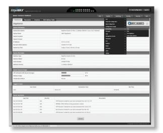
Change the IP Address to a unique IP address or select DHCP on the IPv4 tab. Click Submit.
