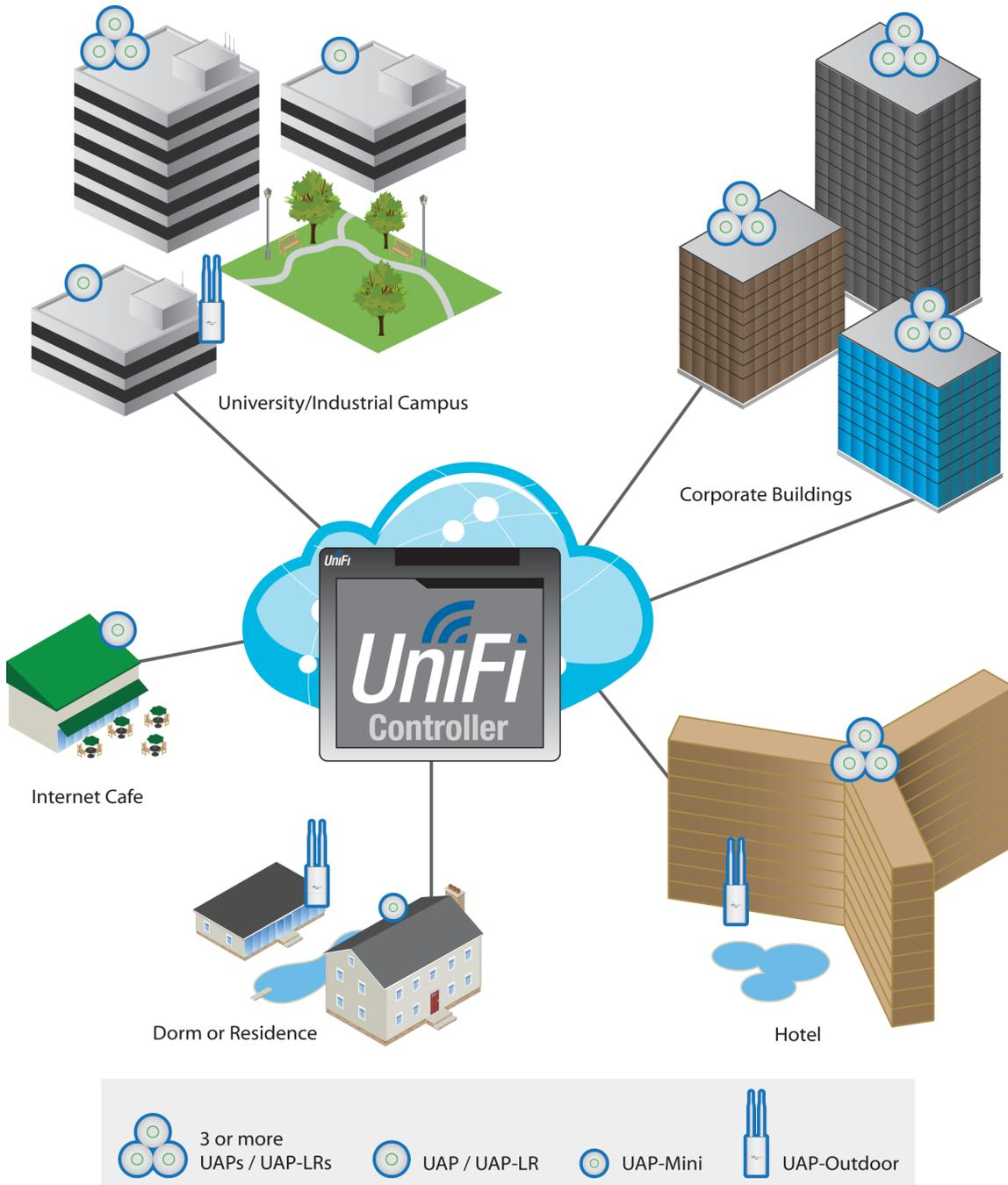
**Extend Wirelessly** Take advantage of wireless downlinking. One wired UniFi AP uplink supports 4 wireless downlinks allowing wireless adoption of devices in their default state and real-time changes to network topology.
