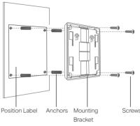
3. Align the mounting bracket and the device, and secure the device into the mounting bracket as shown below.
