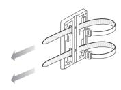
3. Fix the mounting bracket on the pole and fasten the strap, then secure the device into the mounting bracket as shown below.
