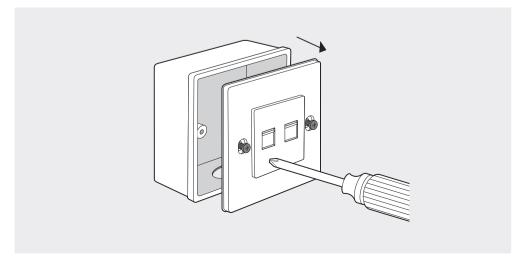
2. Insert the enclosed screws and tighten them with a Philips screwdriver to secure the mounting bracket.
