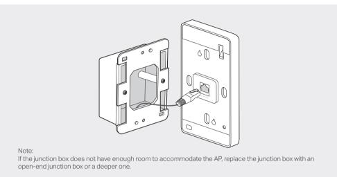
4. Attach the AP to the mounting bracket by aligning the two mounting studs on the mounting bracket with the large opening of the slots on the AP. Press and slide the AP down until it locks into place.
