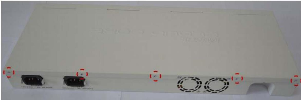
1. Use PH2 screw driver to loose backside screws then side screws, take off cover. Detach DSUB-9 connector fasteners.
