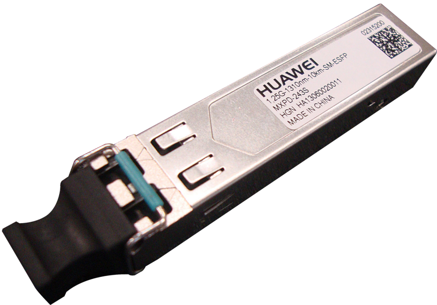
Figure 6-3 SFP/eSFP optical module
