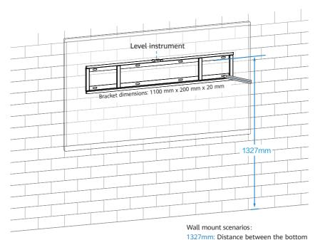
of the bracket upper beam and ground to ensure the optimal angle of view
