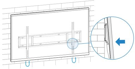
3. If you want to unmount the large screen, take out the pull rope pendants and pull them downwards to open the buckles. You can then lift and unmount the large screen from the wall-attached bracket.
