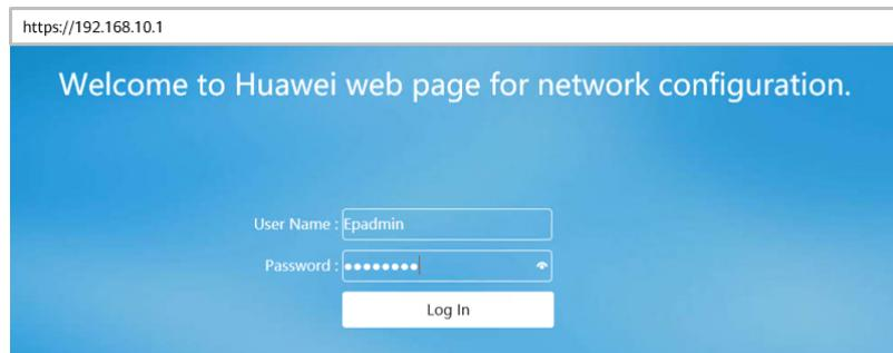
2. Enter the user name and password in the login window. (For the initial user name and password, see the product nameplate.) After the account is verified, you can access the web configuration page.
