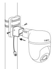
\*Pole-mounting loops are not included. Prepare the required accessories for pole mounting in advance.
