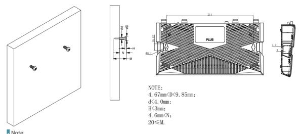
The diameter of the screw head, 4.67mm < D < 9.85mm, and the distance of two screws is 211mm. The screw that project from the wall need around 5mm based, and the length of the screw need to be at least 20mm to withstand the weight of the product.
