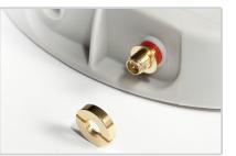
B When installing N-connectors, expand the openings using cutter.
