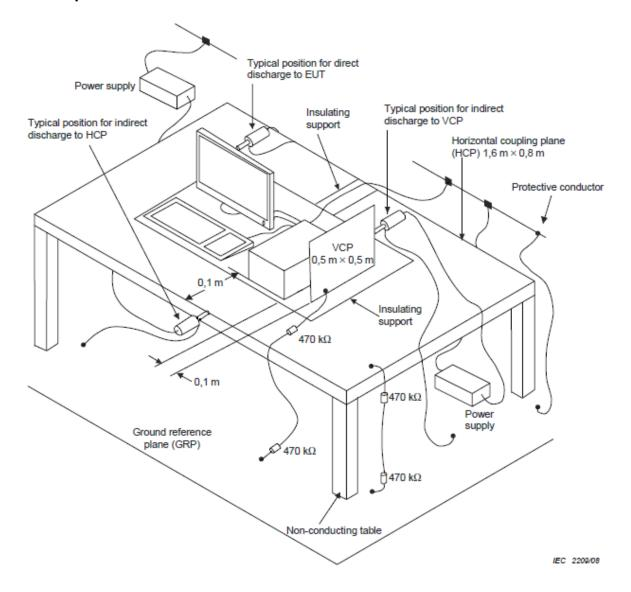
The test setup consists of the test generator, EUT and auxiliary instrumentation necessary to perform DIRECT and INDIRECT application of discharges to the EUT as applicable, in the follow manner: CONTACT DISCHARGE to the conductive surfaces and to coupling plane; AIR DISCHARGE at insulating surfaces.
