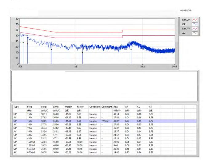
Test Mode Mode 1, LAN Port / 1000Mbps Frequency Range 0.15 MHz to 30 MHz
