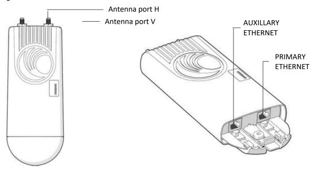
Table 30 ePMP 1000 Connectorized radio interfaces
