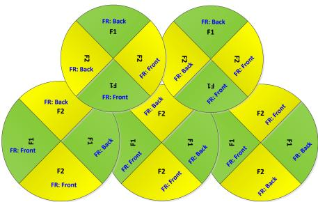
Figure 43 Frequency reuse configuration example
