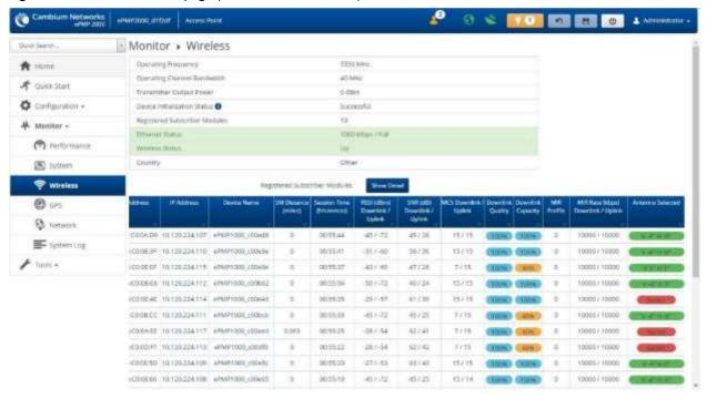
Figure 53 AP Wireless Status page (ePMP 1000 - Detail View)
