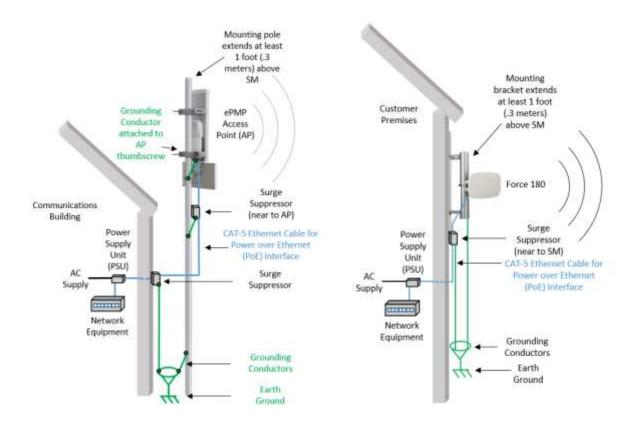
Figure 4 AP Cabling Diagram
