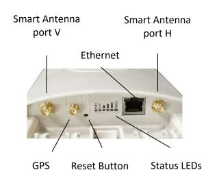
Table 4 ePMP 2000 Access Point with Intelligent Filtering and Sync interfaces
